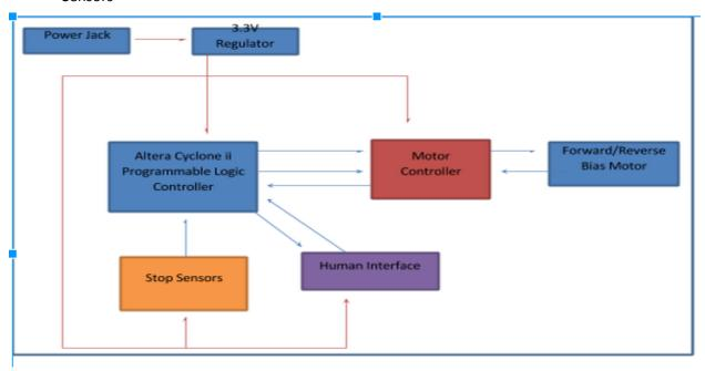
In our design we are using an Altera Cyclone II Programmable Logic Controller which will:
